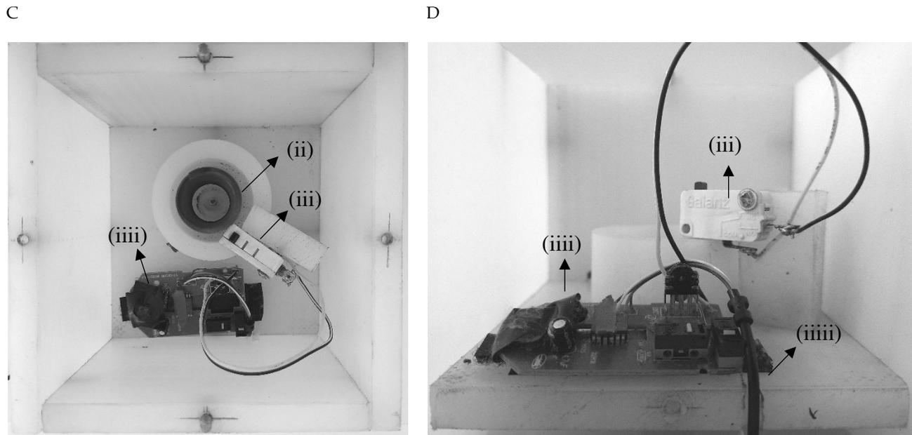
**Figure 2.** Spring Button interior top view on the Panel C and interior side view on the Panel D. (ii) steel spring (the spring is removable); (iii) microswitch; (iii) mouse's circuit board; (iiii) USB cable.
