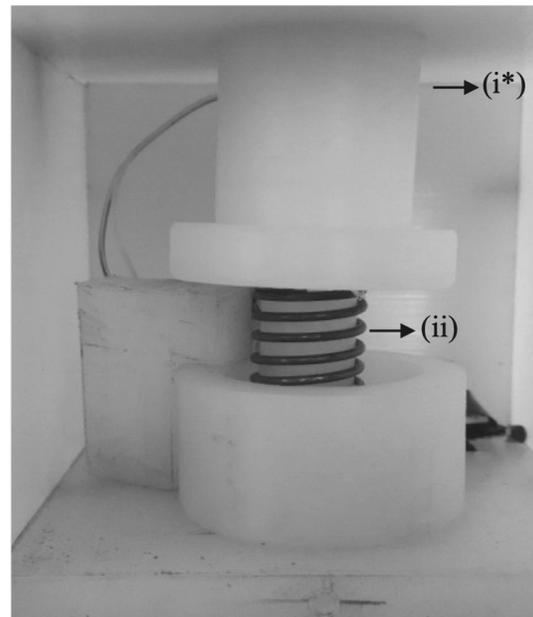
Figure 4. Spring Button's interior side view on Panel E and interior side view with the cylinder pressed down on Panel F. (i) cylinder; (i\*) cylinder pressed down; (ii) steel spring; (iii) microswitch.
